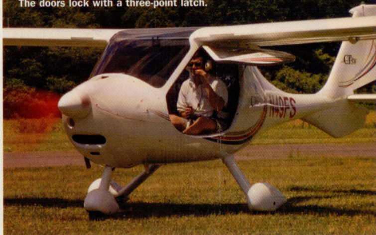
Large, gull-wing doors ease access to the egg-shape cabin. The doors lock with a three-point latch.
